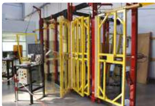
Test for resistance to wear, OTLAV I.U.S.
