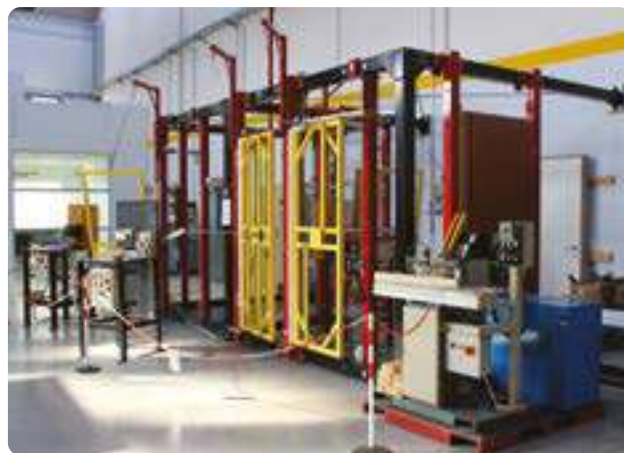
View of the OTLAV test laboratories I.U.S. (Intensive Use Simulator)
