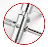
By acting on the threaded pin it is possible to quickly fit the hinge using the appropriate hexagonal bit for electrical drill screwers and then make the side precision adjustment using the special "T" wrench.
