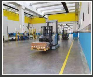
For the transportation of all necessary material, "OAMH" makes use of special automatic trolleys designed and built specifically for OTLAV, called **LGV** (Laser Guided Vehicle). These trolleys transport and distribute the necessary materials to individual machinery for seamless working in a completely automatic way. Speed, safety and precision.
