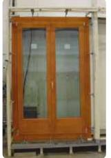
Test for resistance to water and wind (in external laboratories)
