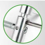
By using a "T" wrench it is possible to adjust the height of the pivot, therefore raising the female part. The weight of the door is evenly distributed over all the door-frame hinges thanks to the great sensitivity of the height adjusting device.
