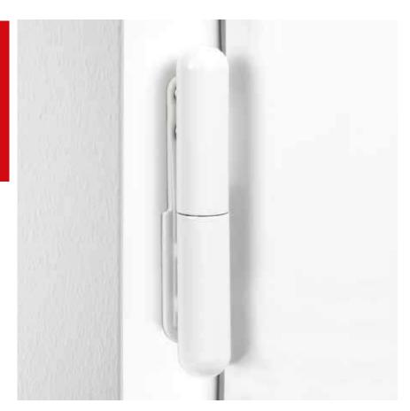
**CE certified** hinge, the door part is suitable to be fitted in the **European groove axis 13 mm or axis 9 mm** with 12 mm clearance. The male part is available with three different types of pegs and two plate models. Discreet, elegant hinge distinguished by ease of installation and **three-dimensional adjustment** with the door fitted. Available in different kind of finishing, suitable for wooden door equipped with European groove.
