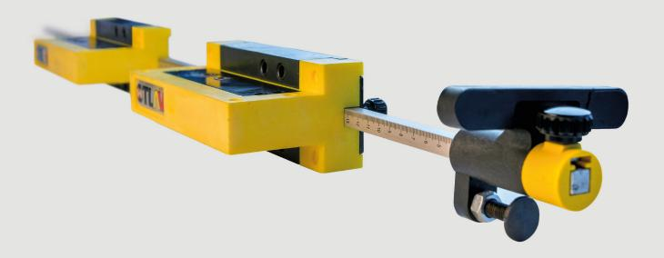
Unlike the standard hinge drilling systems, with MODULAR ROD, thanks to the device which can lodge two or three special tools that permit the separate door and frame drilling for the subsequent hinge fitting, it is not necessary to place the door on the frame; so that it is possible to prepare two separate lines to produce the doors, **that is to say one for producing the shutters and one for the frames.**
