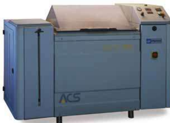
Salt spray chamber: Angelantoni ACS mod. DCTC600.
